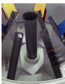
Specimen holder for weathering panels
